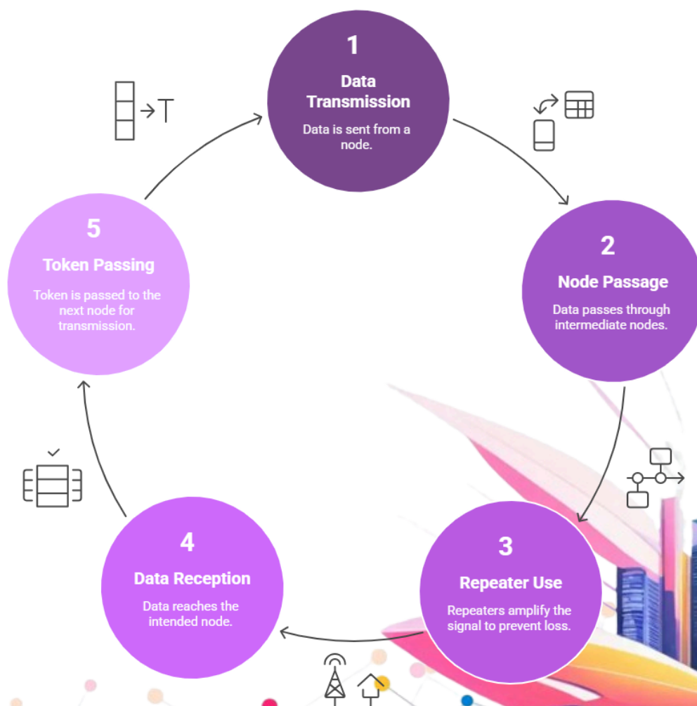
Figure 1.27: Data Transmission Cycle in Ring Topology
